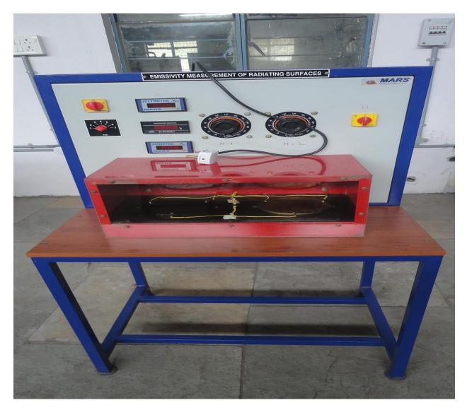
**<u>AIM:</u>** To determine the emissivity of gray surface.
