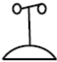
Figure 21.12: Pressure (P) Or Vacuum (V) Actuated Switch , Closes On Rising Pressure - Letter In Symbol
