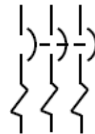
Figure 55: Circuit Breaker with Thermal OI
