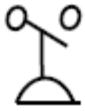
Figure 21.10: Pressure (P) Or Vacuum (V) Actuated Switch , Closes On Rising Pressure - Letter In Symbol
