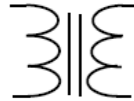
Figure 23: Transformer , Iron Core
