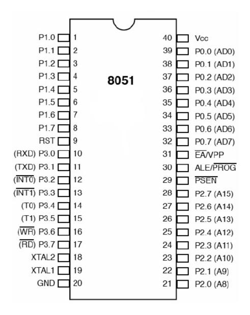
8051 Microcontroller pin diagram
