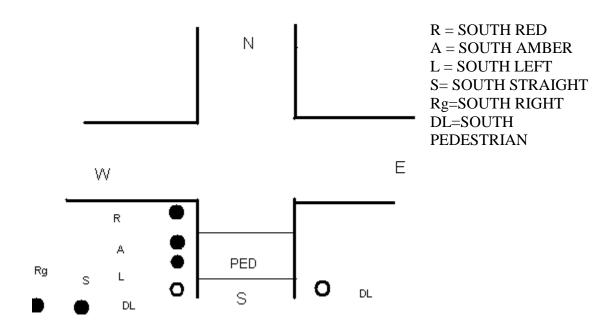
The five LED s (except "Pedestrian") will be ON or OFF depending on the state of corresponding port line LED is ON, if the Port line is Logic 'HIGH' and LED is OFF, if it is at logic 'LOW'. The last LED marked DL is a set of two dual color LED s and they both will be either RED or GREEN depending on the state of the corresponding port line RED if the port line is logic HIGH and GREEN if the port line is logic LOW.
