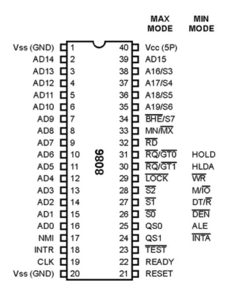
8086 Microprocessor pin diagram
