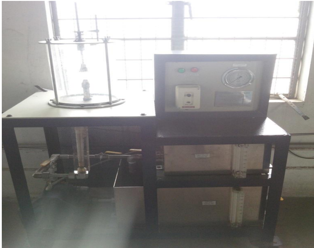
Figure 9. Impact of Jet on Vanes
