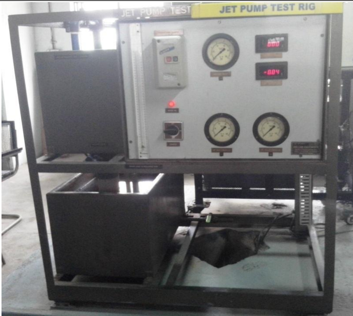
Figure 3 : Jet pump test rig.
