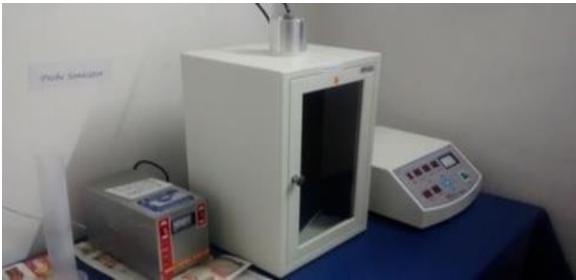
Preparation of CuO Nano fluid using Ultrasonic probe sonicator
