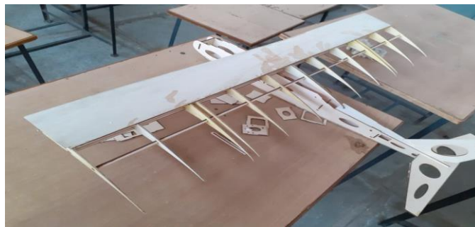
Model in making using Balsa wood with Laser cutting
