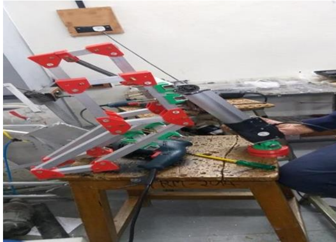
Structural Arm Model with Linear Actuator
