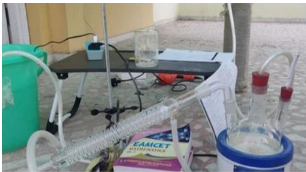
Plastic to Fuel Conversion set up
