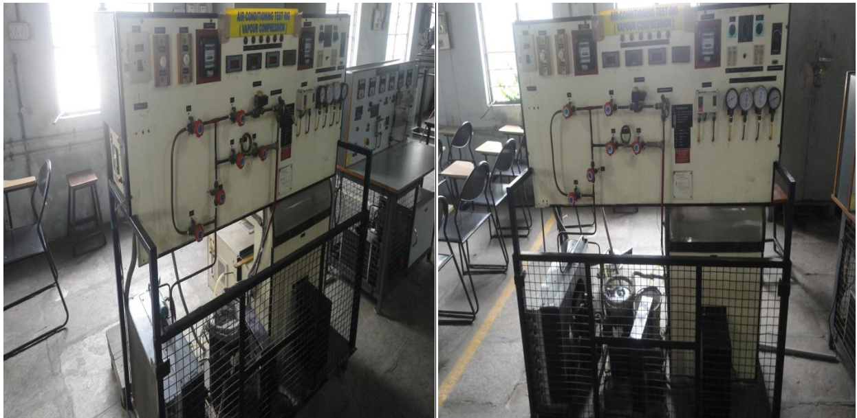
Refrigeration and air conditioning test rig
