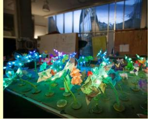
The robotic garden is a tablet-operated system that can be controlled either by a click feature or a code feature where users can use programming techniques to execute their own commands and sequences in real-time. The system includes dozens of fast-changing LED lights and more than 100 origami robots able to crawl, swim and blossom like flowers.
