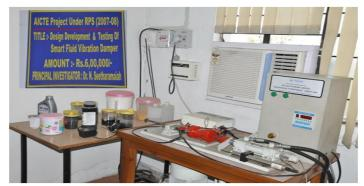
Smart Fluid Vibration Damper set up of MED
