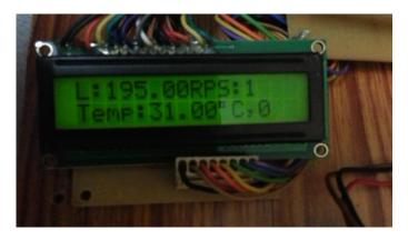
Fig 3 LCD Display showing Level, RPS & Temperature
