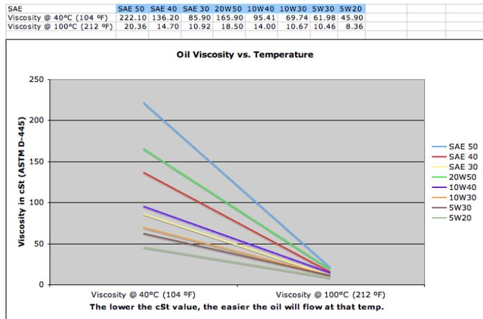
Fig:Variation of Viscosity with Temperature
