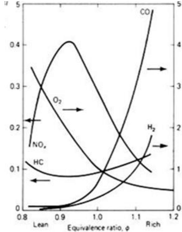
Volume of CO, CO<sub>2</sub>, HC, O<sub>2</sub> and NO<sub>x</sub> for different air fuel ratios / equivalence ratio
