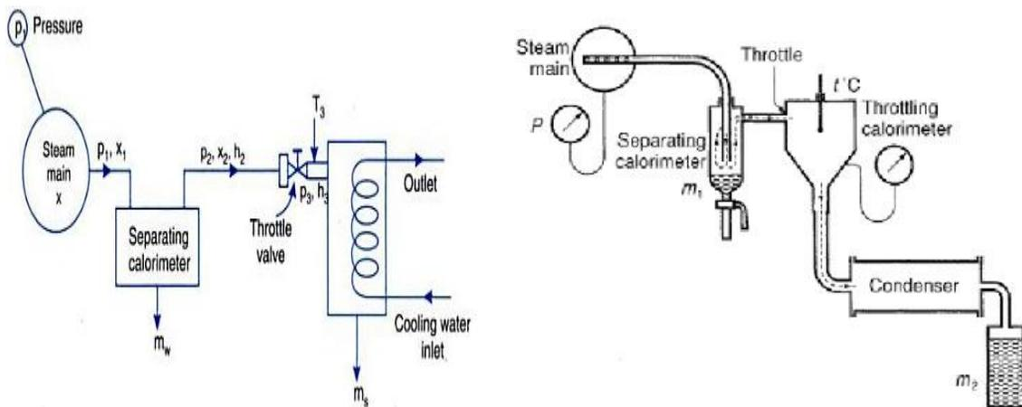
FIG:Line Diagram separating calorimeter
