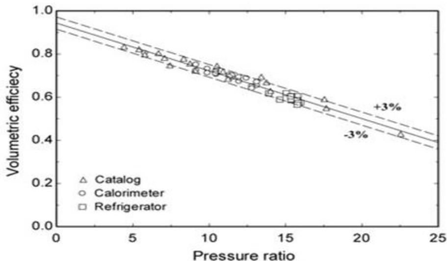
Correlation between the volumetric efficiency and pressure ratio.
