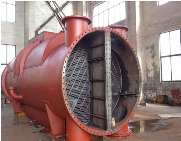
**Straight-tube heat exchanger
