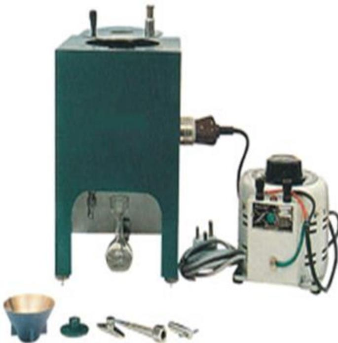
FIG: Say bolt Viscometer
