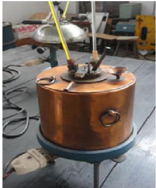
**Description:** Abel's apparatus is used to determine the flash point of light oils and fuels. Fuel Oil is heated indirectly by a hot water bath which surrounds the oil cup. A thermometer shows the temperature of oil and water separately. Test flame is taken near the oil bath frequently to determine the flash point.
