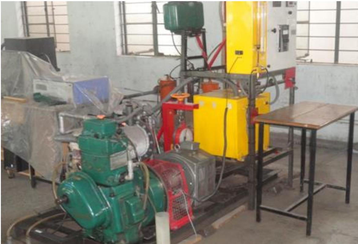
Fig: 4 stroke single cylinder disel engine
