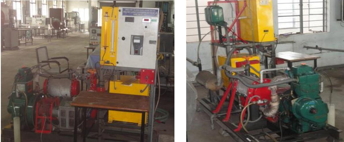
Fig: 4 stroke single cylinder diesel engine
