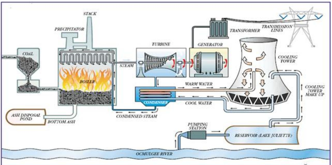
Fig: steam power plant layout
