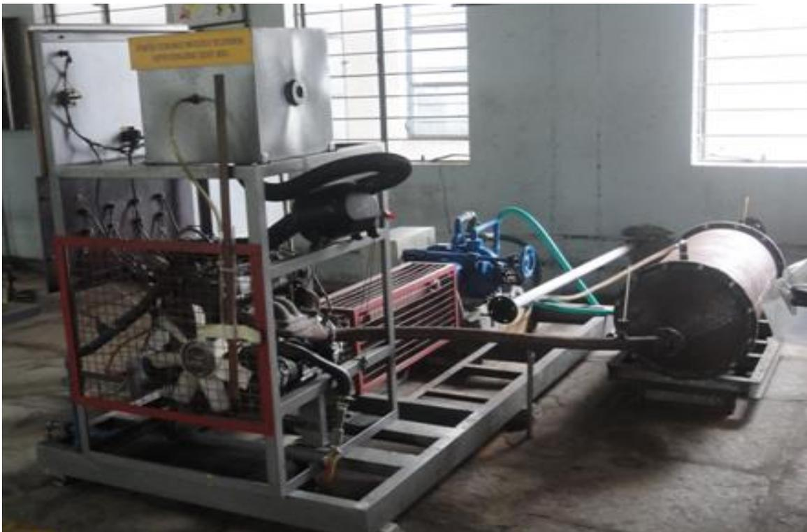
**Fig: 4 stroke 4 cylinder petrol engine (MPFI)**
